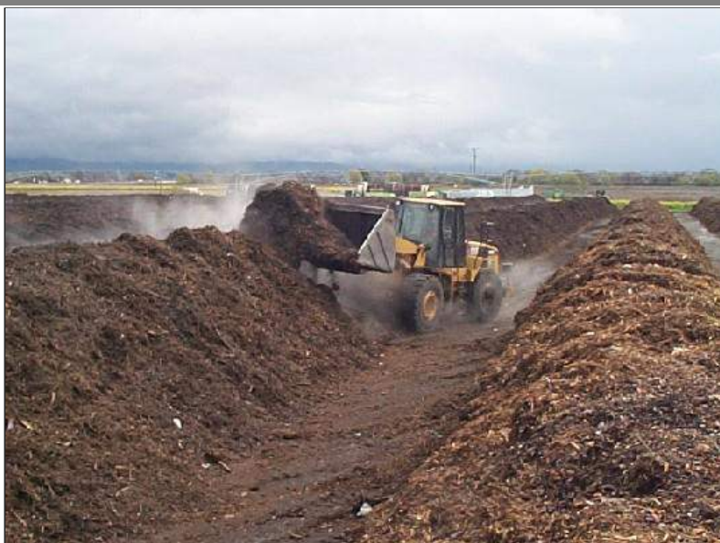
Photo 6-1 Turned Windrow Composting Facility
