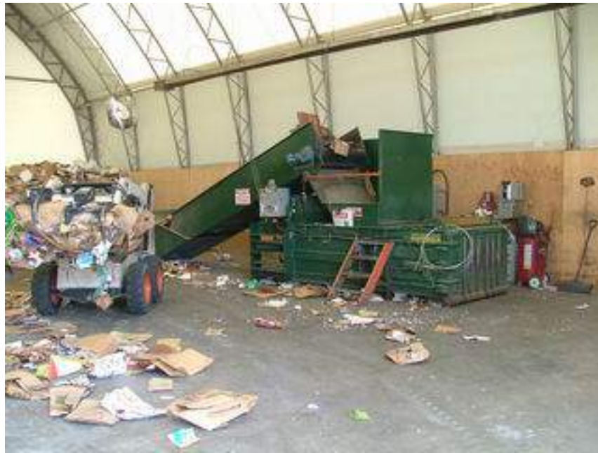
Photo 5-7 Northern Recycling Horizontal Baler
