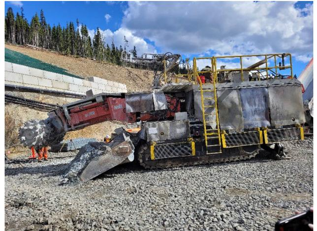
Figure 26: Road header – drill planned to be used instead of blasting for Cariboo Gold where feasible.
